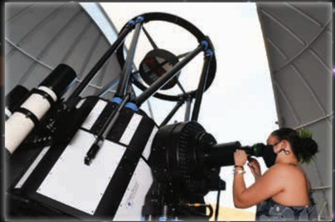
Jaylee Koanui-Nefalar guides guests on the Kilo Hōkū Experience. The PW1000’s telescope dimensions: 135 inches high, 72 inches wide, and 45 inches deep.
