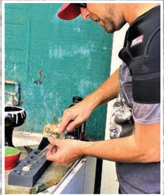
Working glass in the graphite mold
